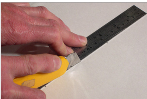
[17] Cut two lines about 1-2 mm apart between the marked points on the left-hand flap and remove the narrow strip of card between the cuts.
